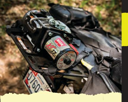
TIP: To transport your winch, WARN offers several bike-specific stow plates. To maintain the option of carrying the winch with Giant Loop Siskiyou panniers, BDCW has the Multi-Function Rear Rack that is pre-drilled to accept the compact F800GS stow plate. This setup keeps the winch far enough back to preserve the area across the panniers for carrying additional gear.
