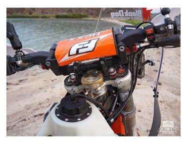
A steering stabilizer is like insurance for nasty surprises: the rock you hit that tries to rip the bars out of your hands, the sand-induced weave you didn't see coming, the sudden head shake from the air blast of a passing semi. Stabilizers smooth out the feedback and help you stay pointed in the right direction. Scotts is an industry leader, and the *BRP SUB* mount fits under the bars, leaving space to mount a GPS or phone up top. They also use the stock handlebar mounts and triple clamps.
