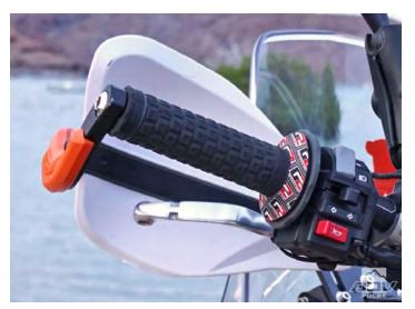
Cold hands add to rider fatigue, so Forgét added grip heaters from *Kimpex*. The inside design allows riders to use whatever grips they prefer. It uses 26.8 watts on the high setting and 21 watts on low, and uses a simple-but-effective rocker switch control.
