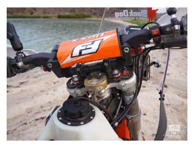
The "flex" part sounds strange, but you can't actually feel any movement in the bars while you ride. What you do feel is a noticeable reduction in vibration thanks to a bushing that eliminates any metal-to-metal contact between the part you grip and the part connected to the handlebar clamps. That means less fatigue and no cramped wrists at the end of a long ride.
