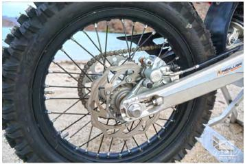
*Galfer's Tsunami* discs are grooved to allow more air flow to the pad, keeping brake temps down and performance consistent. The advantage is twofold: increased braking power and, more importantly off road in slippery conditions, better ability to modulate that power. Forgét coupled them with sintered pads, which are heat resistant and long wearing in a variety of conditions.
