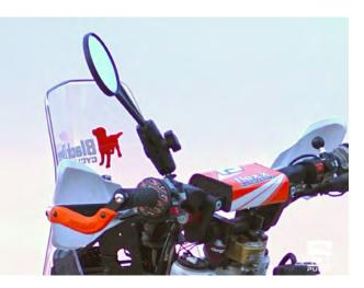
The simple, nearly indestructible design holds steady on the road or trail, thanks to the *RAM Mount* you can crank down hard, and it neatly folds away behind the headlight when the trail gets tight. It will give way instead of break if you fall with it extended, and If you do manage to break the glass part, *Doubletake* sells replacements.
