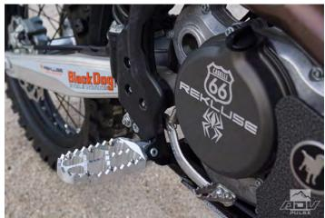
Made out of tough billet aluminum and deeper than stock, the *Rekluse* clutch cover will stand up to abuse and provides a small increase in engine oil capacity, a good thing on a bike that doesn't hold much oil in the first place. The *Kurt Caselli Limited Edition* honors the legacy of the late Baja racer. *Rekluse* donates \$125 from every sale to the *Kurt Caselli Foundation*, which promotes off-road rider safety.
