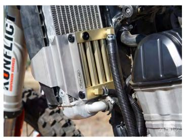
Another clue to the bike's nature is its 1.5-liter oil capacity. That's not a lot, and it means frequent oil changes if you rack up a lot of miles. Forgét addressed this issue by adding a *Twin Air* auxiliary cooler. It bolts on behind the left radiator so it's out of harm's way, keeps oil temps down and increases capacity by 10 percent.
