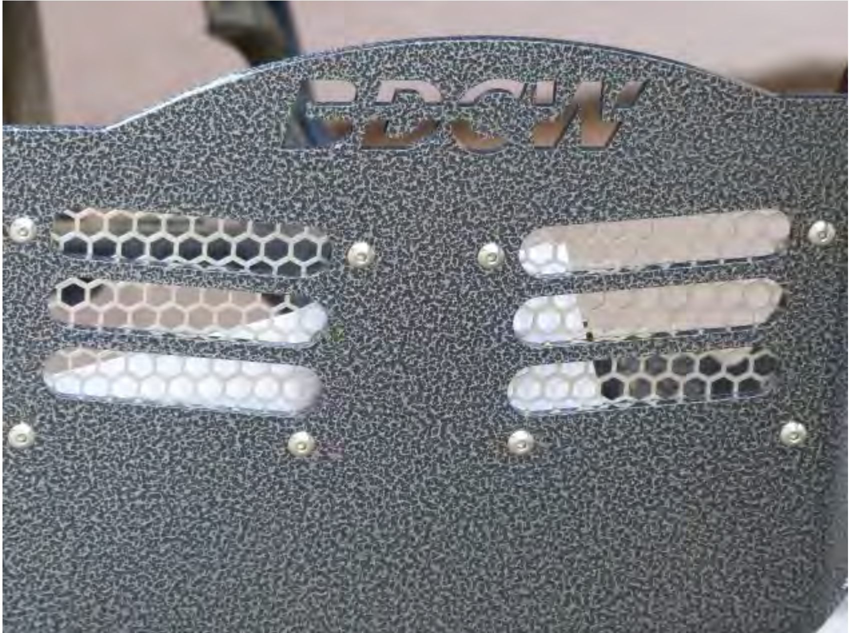
The BDCW Ultimate Skid Plate 2.0 with integrated Side Stand Relocation.
