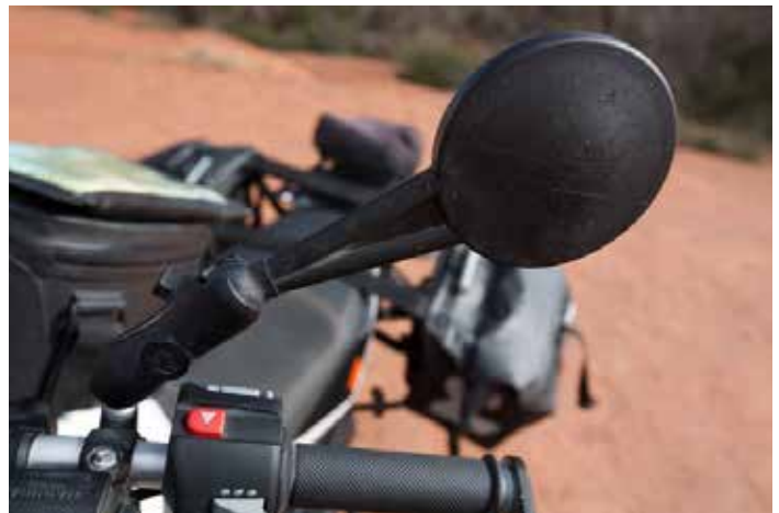
Strong and foldable, these Doubletake mirrors are a wise modification for trail use.
