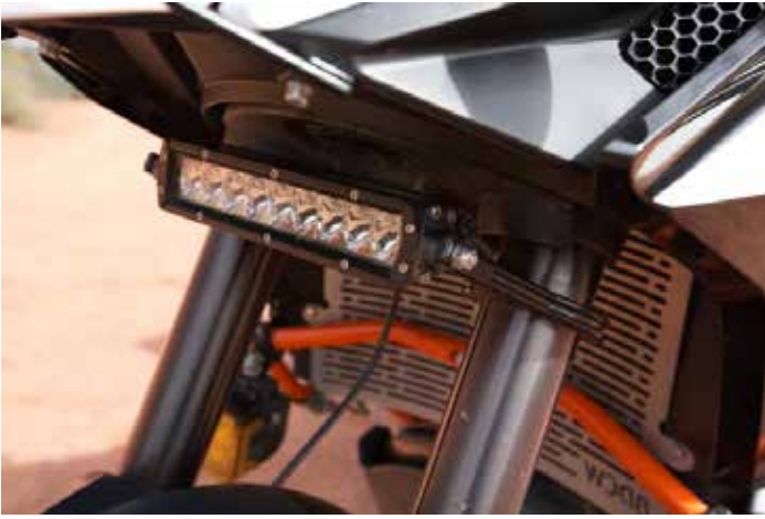
The 6" Rigid LED made night riding an easy affair, aided by the light turning with the front fork.
