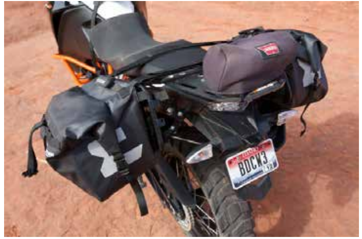
The rear rack runs far back enough to allow a winch mount and still fit a generous top bag.
