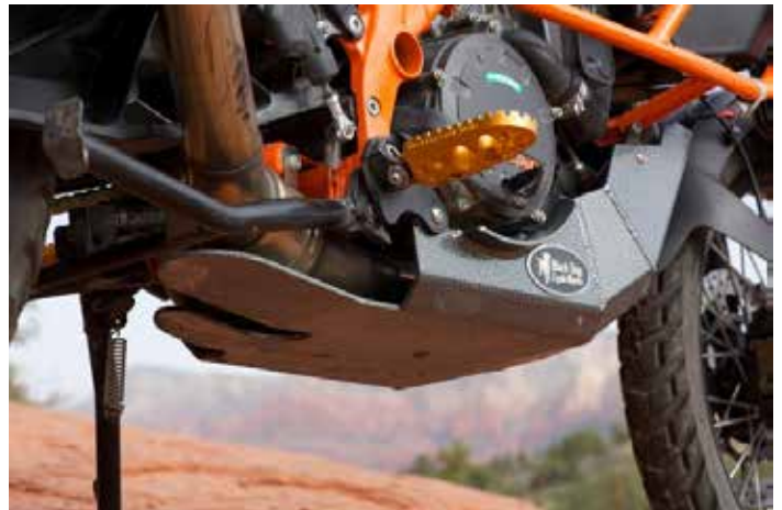
The rear of the plate protects the exhaust and center stand.
