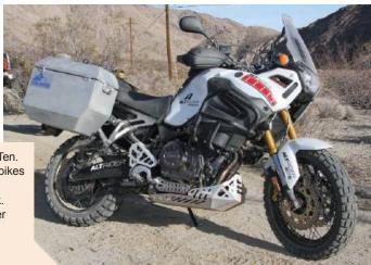
of Jesse hard cases, Clearwater LED lights, a Giant Loop tank bag and Sava tires finished the preparation.
